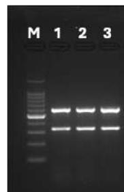
**Detection of PCR products using Agarose Gel electrophoresis:** Lane M: 100 bp ladder. Lanes 1-3: Amplified PCR products electrophoresed on 2% agarose gel (pre stained with 1x eDNAsafe™) in 1x TAE buffer Visualized under UV transillumination.
